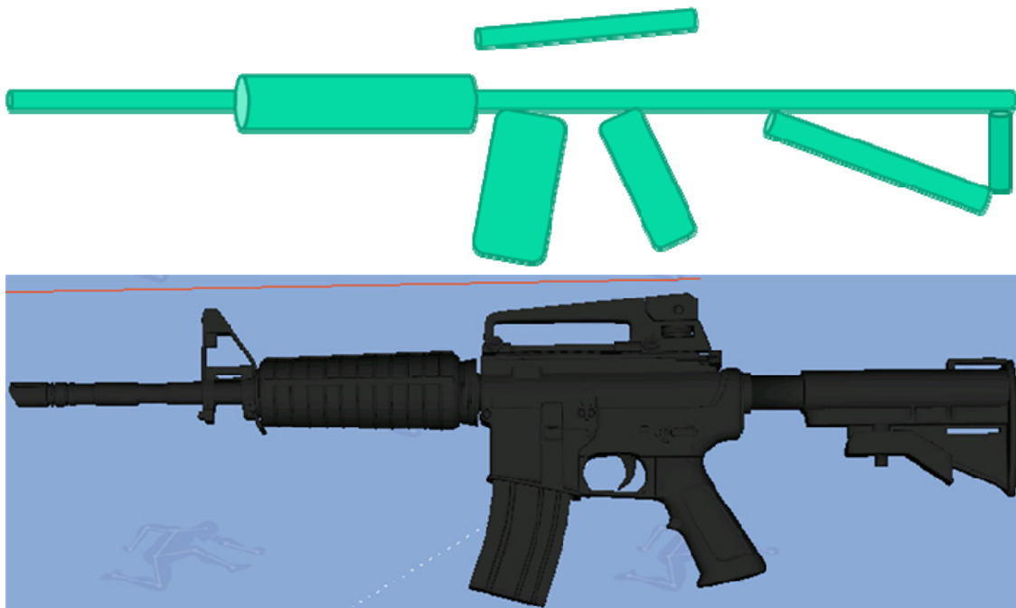
Figure 6.6. Modeling of rifle for collision avoidance with 5 finite cylinders and 2 finite planes
