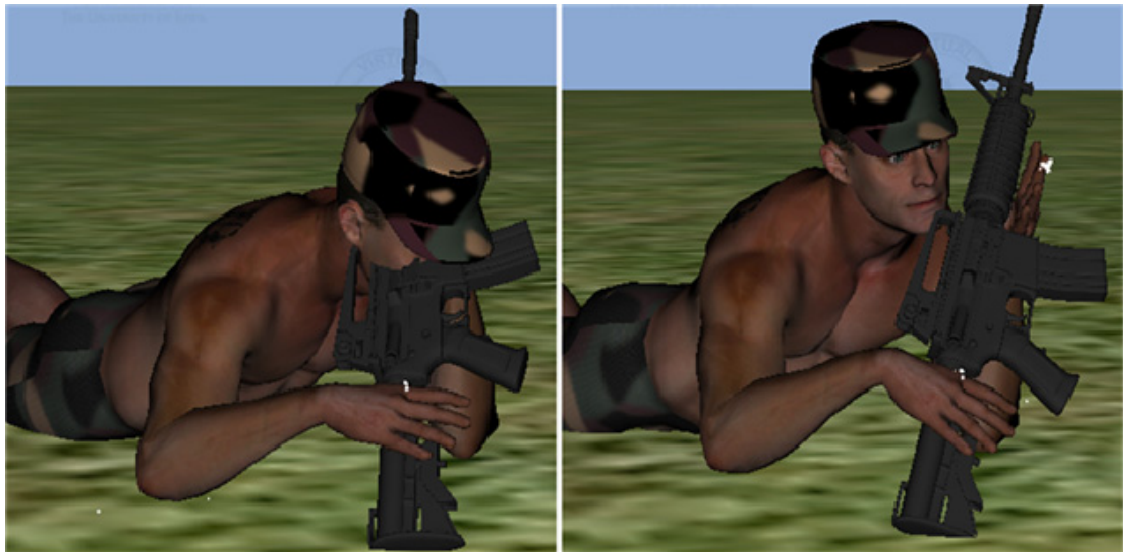
Figure 6.5. Comparison of the results with and without collision avoidance: Collision avoidance constraints change the avatar's motion to prevent the penetration of the rifle with the avatar.
