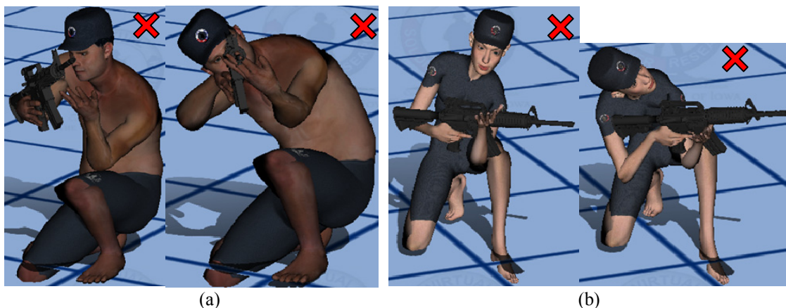
Figure 5.21. Solution of an avatar played on a different avatar intentionally to show the sensitivity of "Kneeling" task to input parameters (a) Solution of "Sophia" incorrectly played on "Santos A" (b) Solution of "Santos A" incorrectly played on "Sophia"
