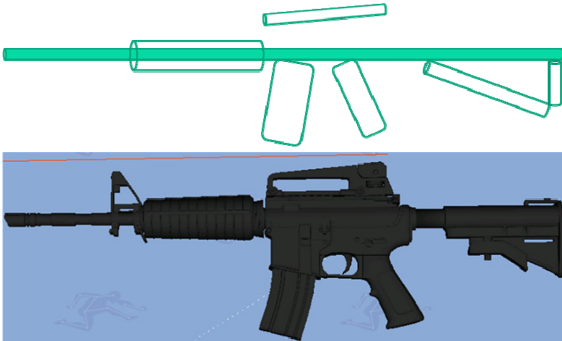
Figure 6.3. Modeling of rifle for collision avoidance with one finite cylinder
